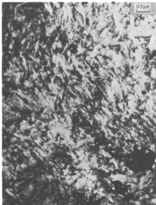
Figure 12 Transmission electron micrograph of Pd–Ag–Cu alloy solution treated at 1133 K, water-quenched and aged 24 h at 673 K showing the discontinuous structure.
